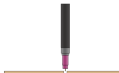
▲ Flat Butt Welding
